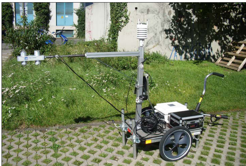
Photo 1 Mobile weather station with multisensor WXT520 (Vaisala), CNR1 radiometer (Kipp and Zonen) and data logger (Campbell Scientific)
