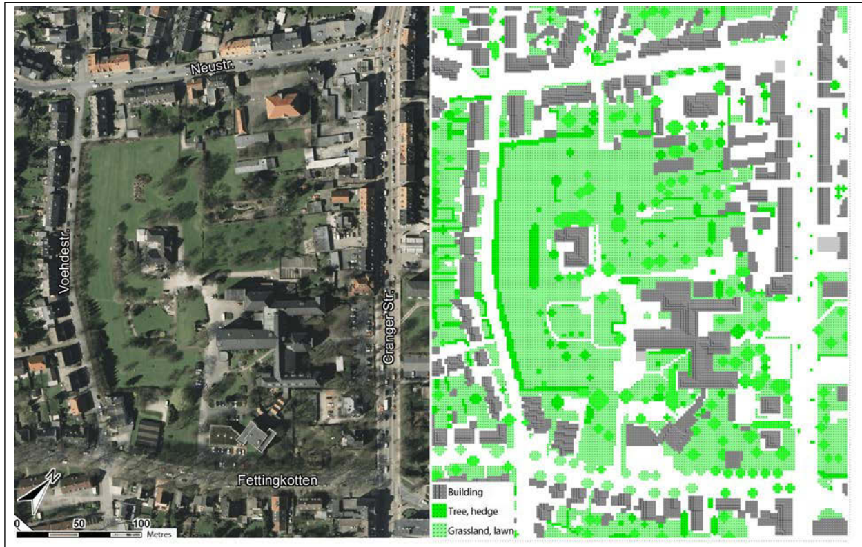
Fig. 2 Aerial photograph (left) and building and vegetation model (right) showing the current situation of the ENVI-met model area "Elisabeth-Stift Erle" in Gelsenkirchen; source of aerial photograph: IT-NRW 2012
