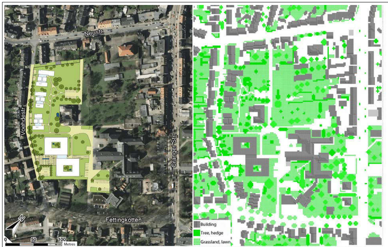
Fig. 3 Aerial photograph (left) and building and vegetation model (right) showing the planned situation of the ENVI-met model area "Elisabeth-Stift Erle" in Gelsenkirchen; source of aerial photograph: IT-NRW 2012
