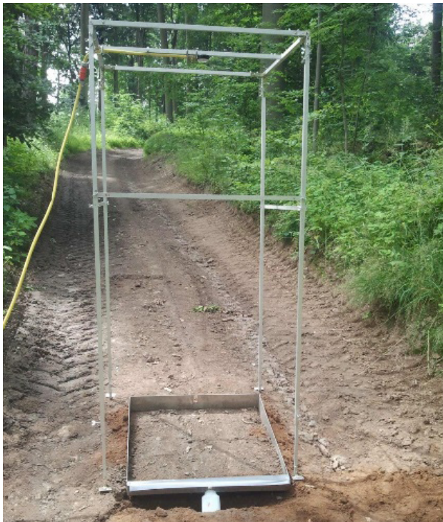
Photo 1 Applied self-constructed nozzle rainfall simulator. Photo credit: Julian Zemke (2016)
